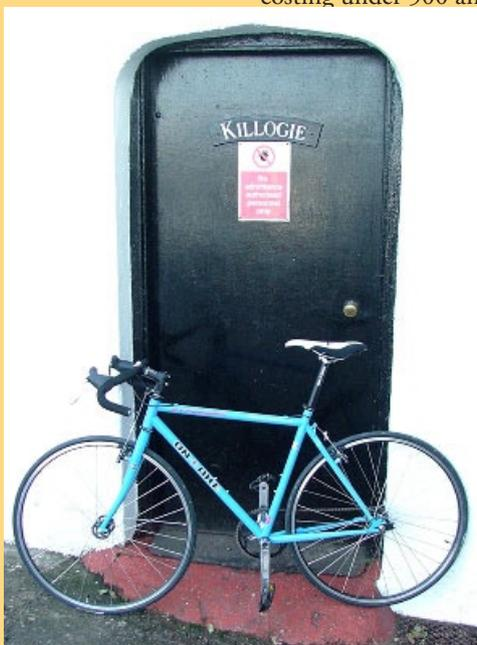
which cost more for the frame than this complete bike. smart thinking employed on the seat clamp which has the slot at the front, keeping much of the rear wheel crap from welding the post to the tube (eventually). considering the bike turned up in two boxes - one for the wheels and one for the frame assembly, the finished item looked 'well smart' as my son would say. just the sort of machine that invited the unwary to take it for a scoot somewhere close by.
